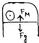
The rod attains the terminal velocity when the magnetic and gravitational force are equal to each other.
